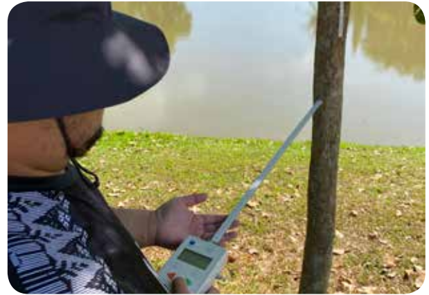
Pengukuran LAI menggunakan alat Ceptometer (AccuPAR LP-80) Measurement of LAI using Ceptometer (AccuPAR LP-80)
